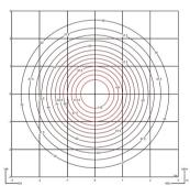
Efficiency Coordinate System 66.69 lm/W CG Total Flux 3103.46 lm Maximum Value 813.96 c
