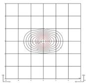
60.85 lm/W Efficiency CG Coordinate System 3472.02 lm **Total Flux** 699.21 cd Maximum Value
