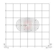
Efficiency Coordinate System Total Flux Maximum Value 60.85 lm/W CG 6944.04 lm 1398.41 cd
