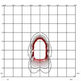
Efficiency Coordinate System Total Flux Maximum Value 31.11% CG 181.22 lm 298.62 cd/klm
