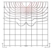
Efficiency Coordinate System Total Flux Maximum Value 108.444 CG 488 lm 1174.12 cd/klm
