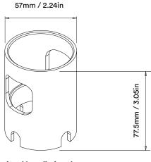
Optional Installation sleeve for screeding and masonry applications only
