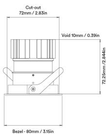
Unit height increases by 21.65mm / 0.85in for spot and elliptical beams
