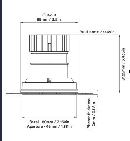
Unit height increases by 21.65mm / 0.85in for spot and elliptical beams
