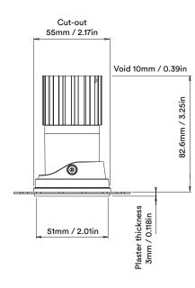
Unit height increases by 12mm / 0.48in for SPOT and both ELLIPTICAL BEAMS
