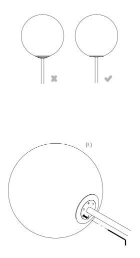
Carefully rotate the Small Glass Sphere 1 (P) onto the Small Male Glass Connector (R1) until the internal location pins are aligned. Gently push the Small Glass Sphere 1 (P) onto the pins until the outside faces of the Small Female Glass Connector (R2) and Small Male Glass Connector (R1) sit flush.
