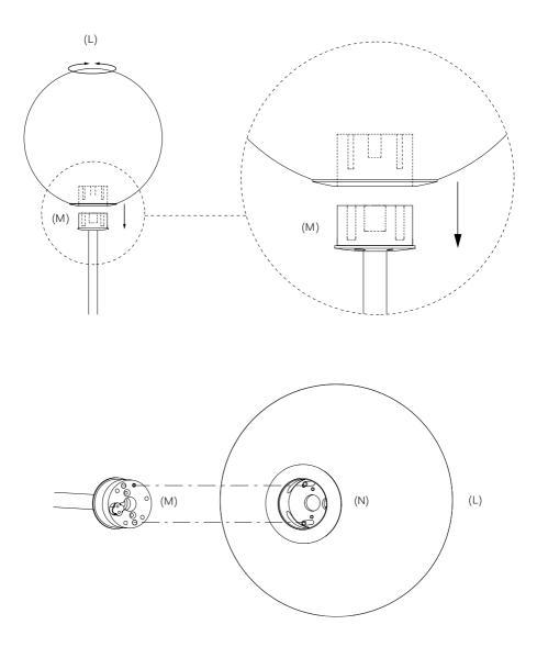
Secure the Large Glass Sphere 1 (L) with the supplied M2×20 screw and hex key, ensuring it is tight to keep the connectors flush.
