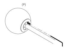
Using gloves, carefully insert the Pendant Rod (S) into the Ceiling Rose (A). Whilst applying upward pressure, gently turn the Pendant Rod (S) clockwise until you feel a small click. This is the clutch engaging. It will feel as if the Pendant Rod has locked but keep gently twisting until it will not twist any further then carefully release the Pendant Rod (S). It will feel like it drops slightly. This is the clutch disengaging and the Pendant Rod will now rotate freely.
