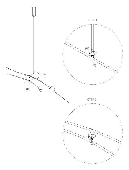
Each joint has a free 360 rotation, allowing the Mobile Chandelier to be positioned according to the space. Lamp Body 1 (M) can rotate freely about the Pendant Rod (S). Lamp Body 2 (Q) can rotate freely about Lamp Body 1 (M).
