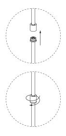
Using gloves, support the Lamp Body 1 (M) and carefully insert the Joint Boss (T) into the Pendant Rod Cap (U). Gently screw them together until tight. Repeat for the Lamp Body 2 (Q).
