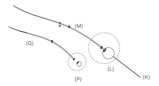
Carefully rotate the Large Glass Sphere 1 (L) onto the Large Male Glass Connector (M) until the internal location pins are aligned. Gently push the Large Glass Sphere 1 (L) onto the pins until the outside faces of the Large Female Glass Connector (N) and Large Male Glass Connector (M) sit flush.
