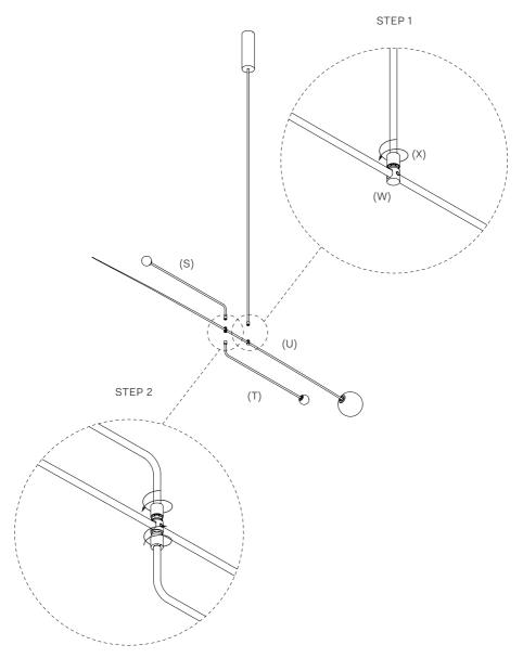
Each joint has a free 360 rotation, allowing the Mobile Chandelier to be positioned according to the space. Lamp Body 1 (U) can rotate freely about the Pendant Rod (W). Lamp Body 2 (S) and Lamp Body 3 (T) can rotate freely about Joint (Y).
