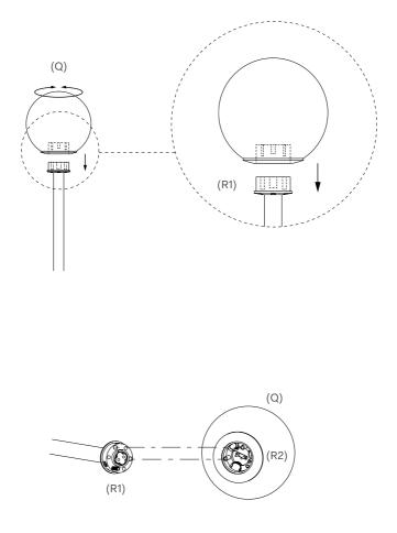
Secure the Small Glass Sphere 1 (Q), with the supplied M2×8 screw, ensuring it is tight.
