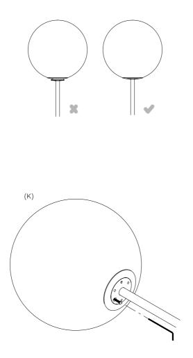
Carefully rotate the Small Glass Sphere 1 (Q) onto the Small Male Glass Connector (R1) until the internal location pins are aligned. Gently push the Small Glass Sphere 1 (Q) onto the pins until the outside faces of the Small Female Glass Connector (R2) and Small Male Glass Connector (R1) sit flush.
