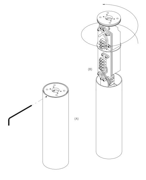
Using the supplied hex key, loosen the four screws attaching the Ceiling Plate (C) to the Ceiling Bracket (B). Slide the Ceiling Plate (C) away from the Ceiling Bracket (B).
