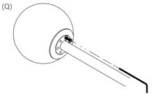
Using gloves, carefully insert the Pendant Rod (W) into the Ceiling Rose (A). Whilst applying upward pressure, gently turn the Pendant Rod (W) clockwise until you feel a small click. This is the clutch engaging. It will feel as if the Pendant Rod has locked but keep gently twisting until it will not twist any further then carefully release the Pendant Rod (W). It will feel like it drops slightly. This is the clutch disengaging and the Pendant Rod will now rotate freely.
