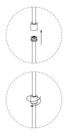
Using gloves, support the Lamp Body 1 (U) and carefully insert the Joint Boss (W) into the Pendant Rod Cap (Y). Gently screw them together until tight. Repeat for the Lamp Body 2 (S) and Lamp Body 3 (T).
