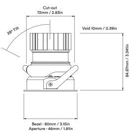
Unit height increases by 21.65mm / 0.85in for spot and elliptical beams
