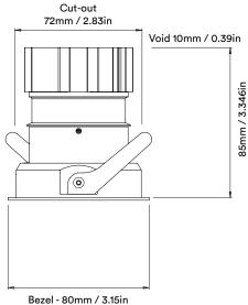
Unit height increases by 21.65mm / 0.85in for spot and elliptical beams
