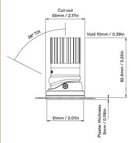
Unit height increases by 12mm / 0.48in for SPOT and both ELLIPTICAL BEAMS
