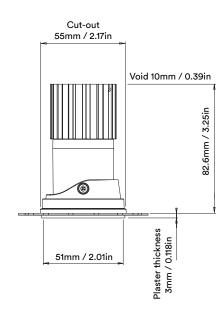
Unit height increases by 12mm / 0.48in for SPOT and both ELLIPTICAL BEAMS
