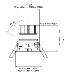
Unit height increases by 21.65mm / 0.85in for spot and elliptical beams
